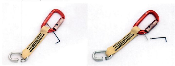
2. Using the included 5/64" hex wrench, remove the set screw and keeper pin from the carabiner in the original tether. Occasionally the keeper pin gets pressed in fairly tightly, so you may need to loosen it with pliers to remove it. **Be careful not to lose the screw or pin!**
