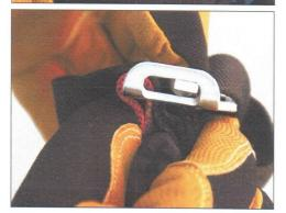
With access to the buckle, move the friction bar in all directions—up, down, side-to-side and diagonally—to ensure it does not separate from the buckle frame.
