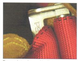
The manufacturer's name (identified as PenSafe or PS) and three-digit manufacturing code will be covered. Push web to the side to reveal the stamped markings.
